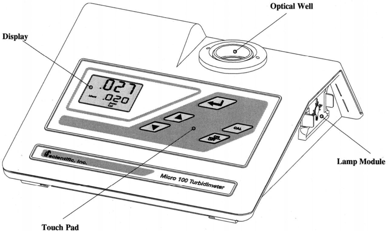
The user interface of the MICRO 100 has been designed with a 5 key touchpad and user display. The five keys of the Touch Pad and their functionality are described below:
