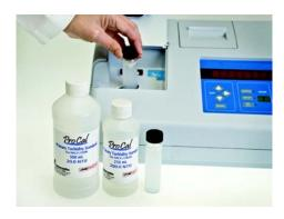
Standards certified \* for use with the Hach® Company's 2100AN turbidimeter. Hach® 2100AN Laboratory Turbidimeter
