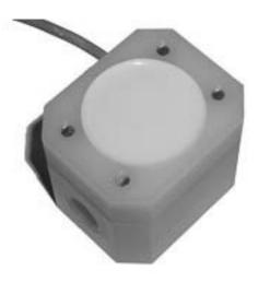
The oval gear flow sensors F3.80 has been designed following the main industrial application requirements: high mechanical resistance and reliable performances. These sensors are suitable to measure a wide range of liquid viscosities with a very high accuracy and repeatability. The sensors can be fixed to flexible or rigid pipes via ¼" GAS threaded process connections. The construction materials, ECTFE (Halar®) or PP or Stainless steel, provide high strength and chemical resistance.
