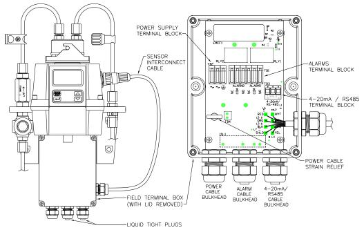
**Figure 5: Electrical Connections for the Instrument**
