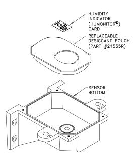
Note: Once the bag is opened, install the desiccant pouch immediately to prevent premature degradation of the desiccant.
