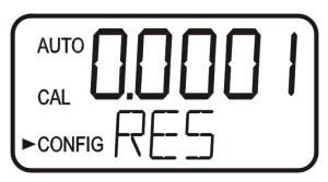
Change the resolution by pressing the  $^{\wedge}$  or  $^{\vee}$  button. When the desired digit resolution has been selected, press the  $\rightarrow$  button.
