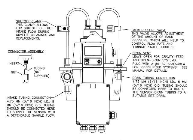
Figure 4: Recommended Plumbing for the Instrument
