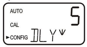
The current selected number of seconds will be shown. Select the desired delay off time for this alarm using the ▲ and ▼ buttons. Once the desired delay time has been set, press the → button to accept it. After the settings for alarm 1 have been completed, prompts will allow for the set up of the information on alarm #2.
