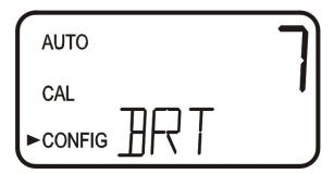
Change the brightness by pressing the  $\triangle$  or  $\nabla$  button. When the desired brightness has been selected, press the  $\bot$  button.
