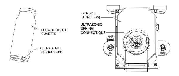
Figure 6: Operational parts of the Ultrasonic Cleaning System
