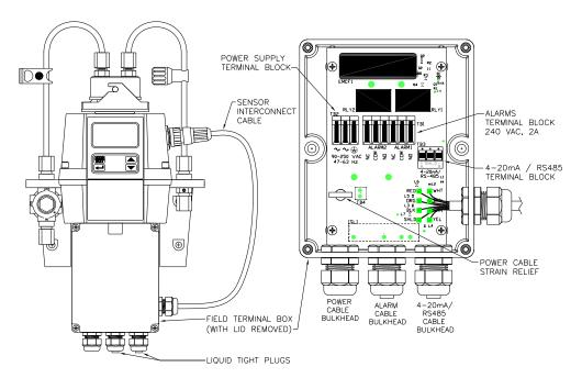
Figure 5: Electrical Connections for the Instrument
