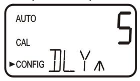
The current selected number of seconds will be shown. Select the desired number of seconds for the "delay on" time for this alarm using the ▲ and ▼ buttons. Once the desired delay time has been set, press the → button to accept it.
