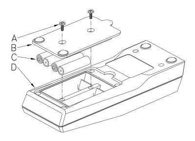
Figure 3: Detailed view of the battery compartment
