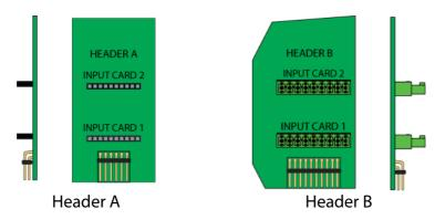
Insert the required input cards between the headers as shown in the following two diagrams, ensuring that the connectors are correctly aligned with the headers on the input cards.
