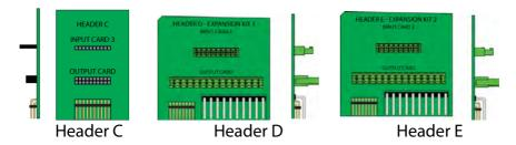
Insert the required input card or output option card between the headers as shown in the following two diagrams, ensuring that the connectors are correctly aligned with the headers on the cards.
