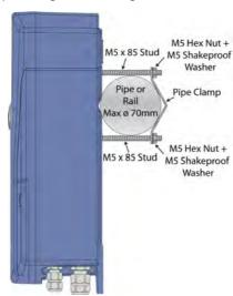
Note: Care should be taken not to over tighten mounting, as damage may result to enclosure.
