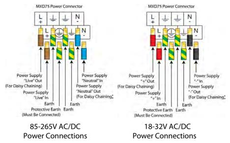
The power supply should be taken from an isolated spur and fused to a maximum of 3 Amps. If the relays require greater current, then a separate 5A fuse will be required. The incoming Earth connection must be connected to the "Protective Earth" terminal.
