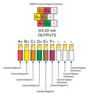
MXD75 Surface Mount Current Output Connection Detail.
