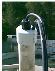
Slip on Cap for Easy removal and insertion of probe
