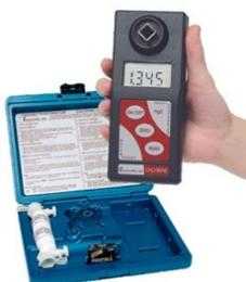
**Chlorine Pocket Photometer - Instrument**
