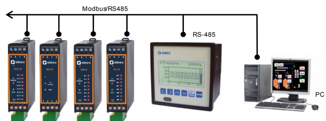
SCADA system with local display
