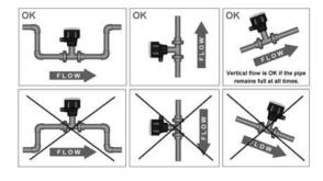
In gravity-flow systems the connection to the tank must be designed so the level does not drop below the outlet: this to avoid pipe to draw air in from the tank causing an erratic measurement of the Magmeter.
