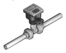
The compact mounting kit F9.KC1 includes the compact plastic adapter with gasket for IP65 watertight installation, the compact cap, the locking ring and four fixing screws for mounting the monitor directly onto the sensor. The instrument and the kit can be ordered separately (code F9.0X.L for the monitor and
