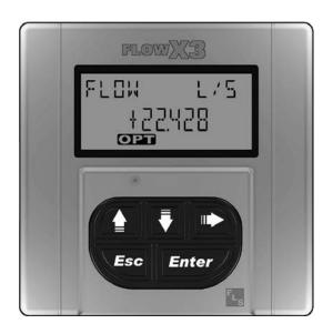
The FLS FLOWX3 F9.00.BD Flow Monitor and Transmitter is designed to convert the signal from the bi-directional flow sensors (F111.HT.BD & F3.11.H.BD) into a display indication and a 4-20mA signal for long distance transmission and it also perform a fully programmable Open Collector digital output. Only one packaging for panel or wall installation makes the device very flexible.
