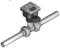
The compact mounting kit F9.KC1 includes the compact plastic adapter with gasket for IP65 watertight installation, the compact cap, the locking ring and four fixing screws for mounting the batch controller directly onto the sensor. The instrument and the kit can be ordered separately (code F9. 5X.L for the controller and code F9.KC1 for the kit) or together using code F9. 5X.XX.L.
