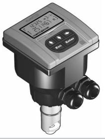
FLS FLOWX3 F9.00 Flow Monitors & Transmitters are designed to convert the signal from all FLOWX3 flow sensors into a display indication and a 4-20 mA signal for long distance transmission. A very simple and complete choice of options are granted by single or dual input/output, two solid state relays output and one relay output.
