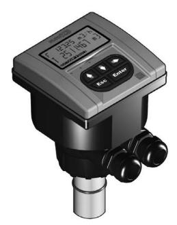
The FLOWX3 F9.60M & F9.63M Insertion Magmeters are suitable to measure flowrate in both metal and thermoplastic pipelines. No moving mechanical parts and the high quality materials allow the measurement of liquids where suspended solids can be present or of abrasive liquids as long as they are conductive and homogeneous.
