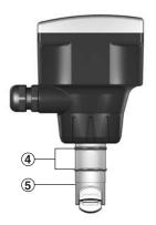
Sensor for compact installation (F3.01) with field-mount transmitter (sold separately)
