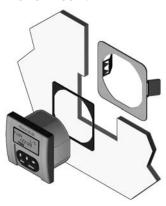
The panel mounting version consists of the monitor and the mounting bracket kit F9.KP1.2 with gasket for IP65 watertight panel installation. The monitor perfectly fits into a standard ¼ DIN panel cutout. The instrument and the kit can be ordered separately (code F9.0X for the monitor and code F9.KP1.2 for the mounting bracket) or together using the code F9.0X.P1.
