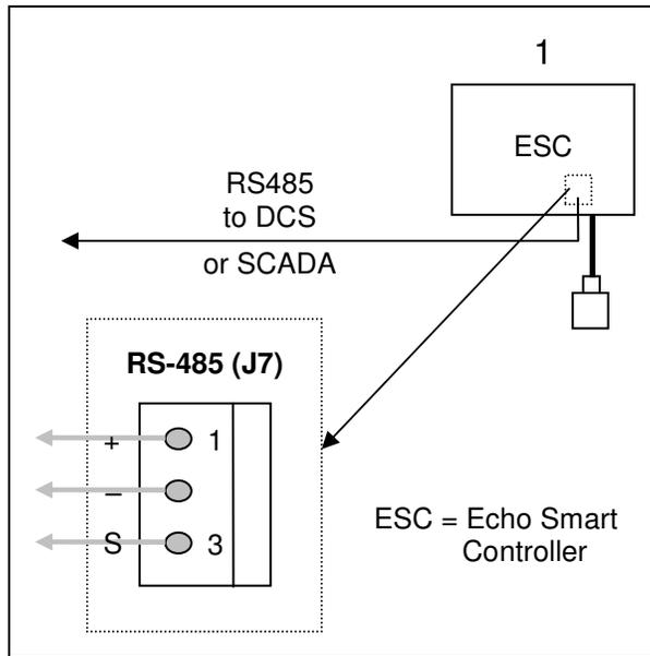
Figure 8.1: Controller with Single Sensor
