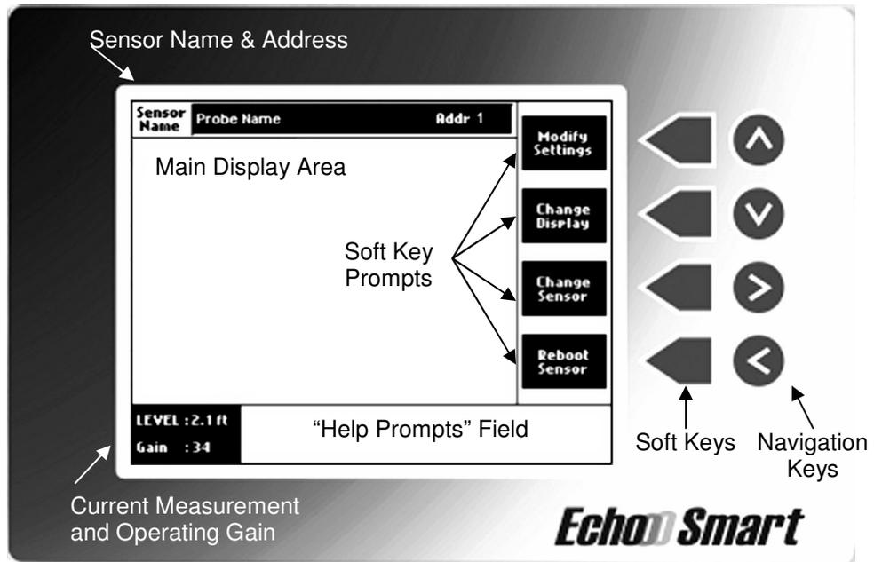
Figure 4.1: The LCD Display
