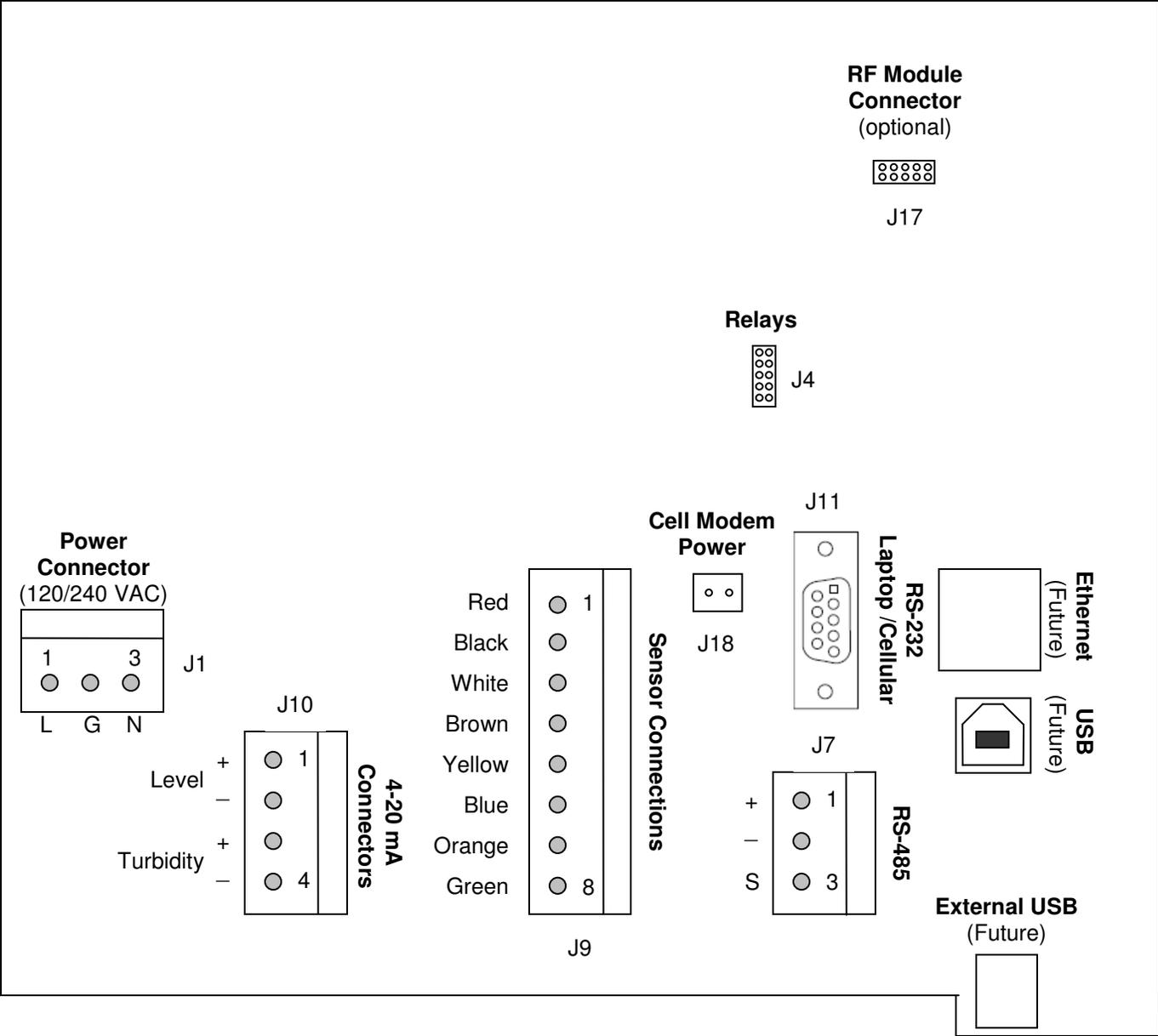
Figure 4.2: Connections for Controller
