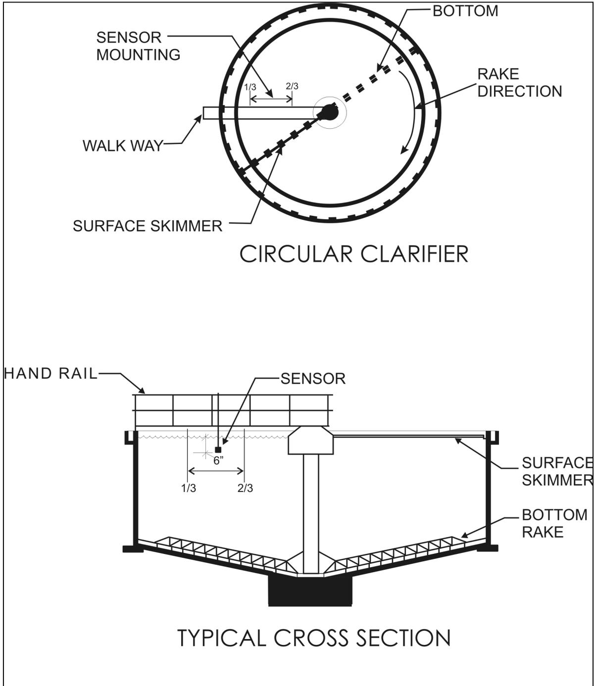
Figure 6.2: Typical 1/3 – 2/3 Location in Circular Clarifier
