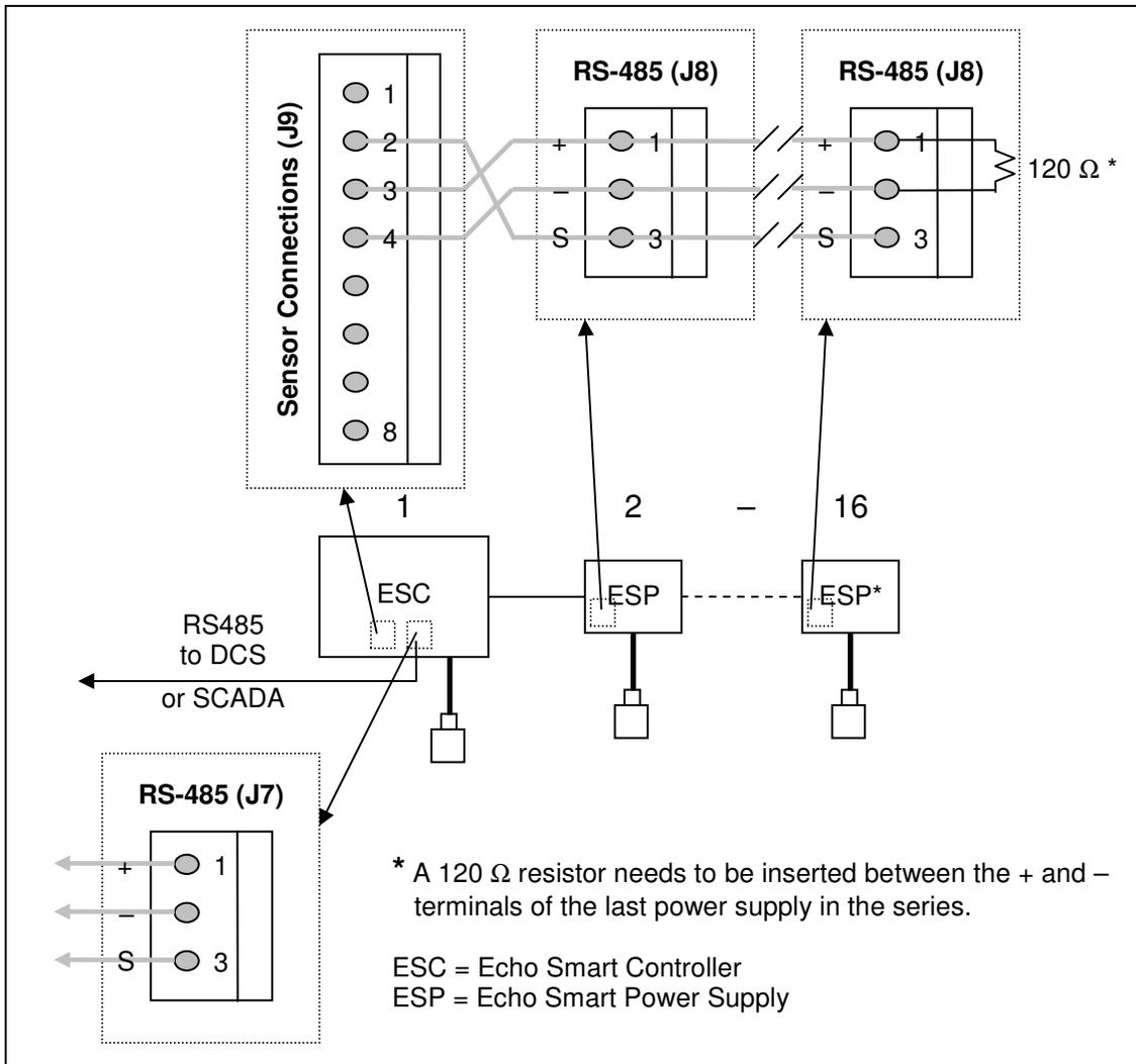
Figure 8.2: Single Wired Field Network
