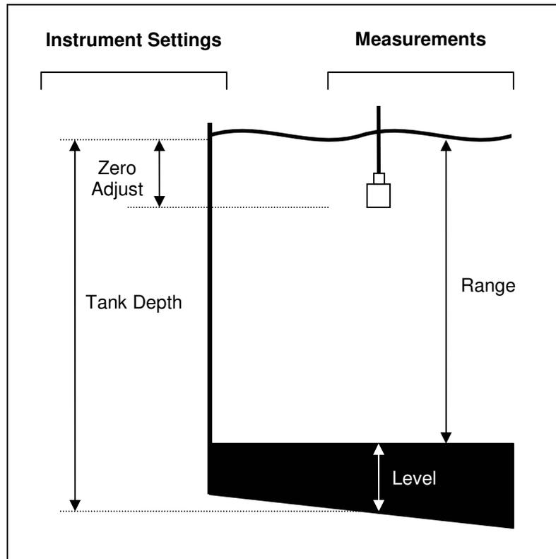
Figure 7.1: Tank Configuration
