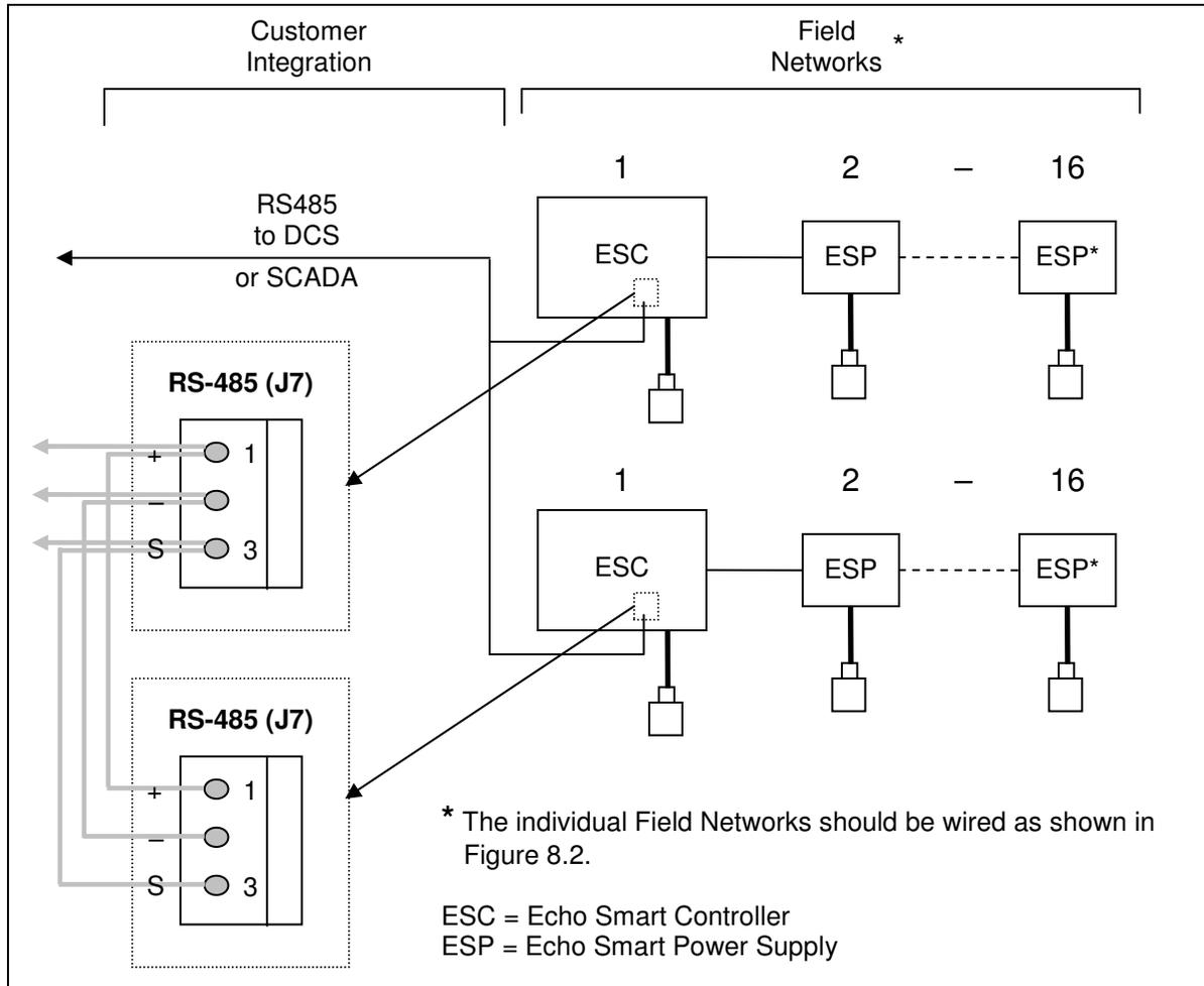
Figure 8.3: Integrated Wired Field Network
