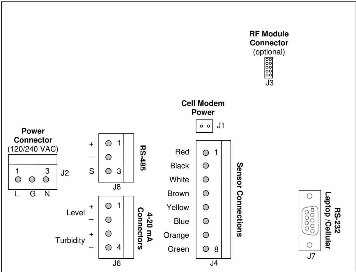
Figure 5.1: Connections for Power Supply
