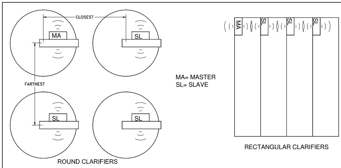
Figure 10.2: Radio Layout Recommendations
