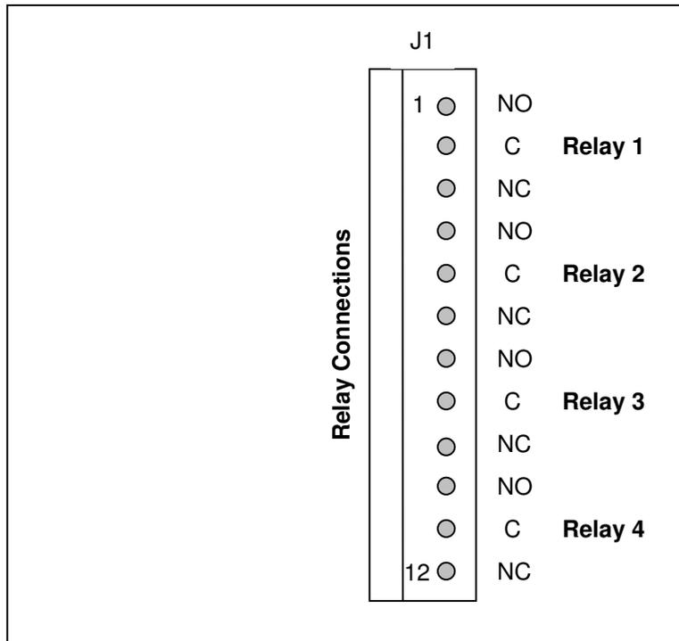
Figure 11.2: Connections for Relay Board
