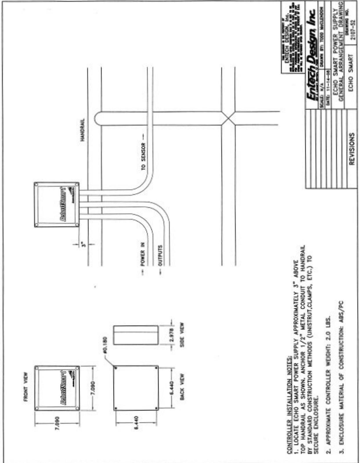
Figure 6.5: EchoSmart Power Supply Unit Installation Drawing
