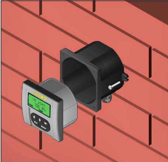
1. Fix the wall mounting kit to a solid wall using the included screws.
