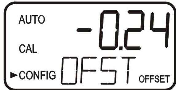
7. If the option was turned **On**, the upper row will display the offset required. This will add or subtract the value of the offset to the measured NTU value. As an example if the Micro TOL measures the process at 0.16 NTU but the laboratory instrument read the sample at 0.12 NTU, adding an offset of  $-0.04$  would result in the Micro TOL displaying 0.12 NTU.
