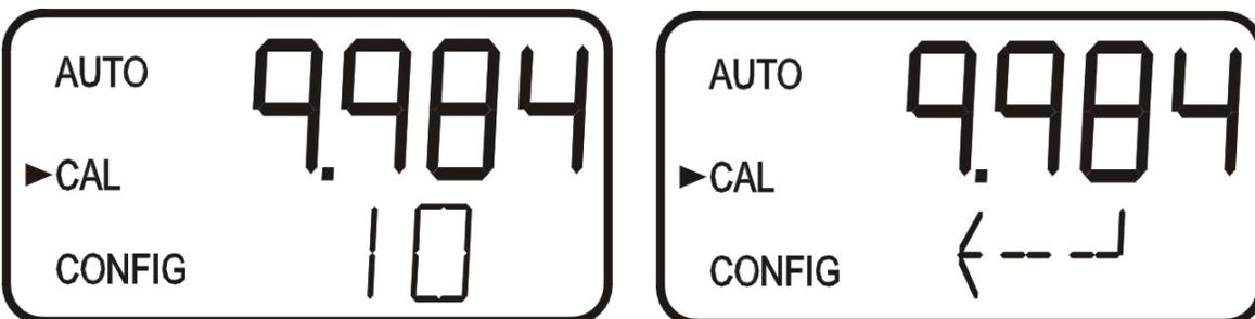
7. If the alternating **10** and  $\downarrow$  is not displayed, push the  $\uparrow$  or  $\downarrow$  until this display is shown.
