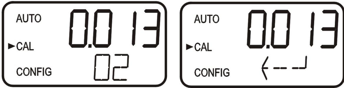
12. Insert the requested 0.02 NTU standard. Index the standard to the lowest value on the upper display.
