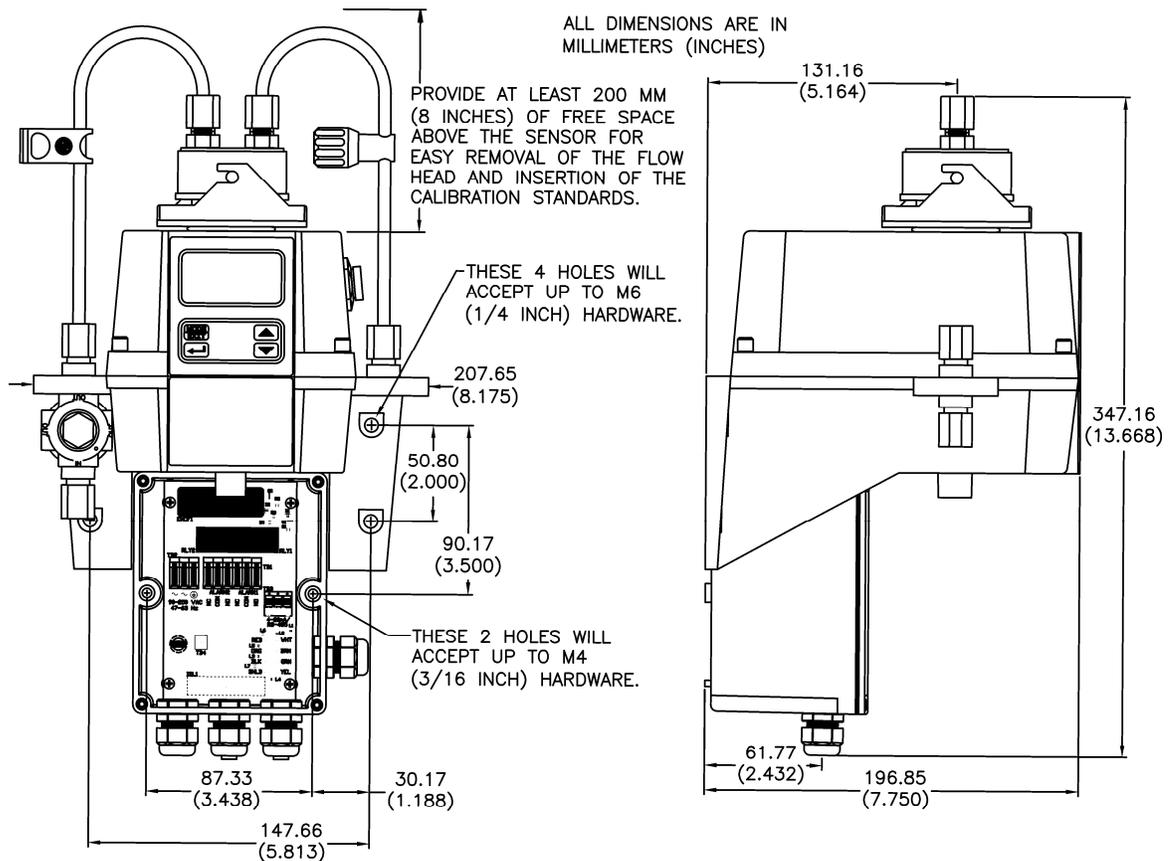
**Figure 3: Overall Mounting Dimensions of the Instrument**
