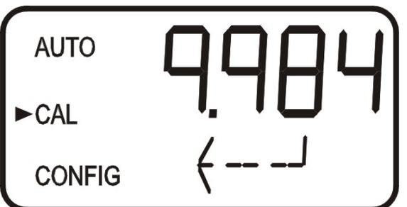
7. If the alternating **10** and  $\downarrow$  is not displayed, push the  $\uparrow$  or  $\downarrow$  until this display is shown.
