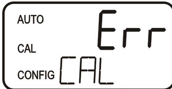
To recalibrate press the MODE key and start the calibration sequence again. To restore the factory calibration, push and hold the ▲ button. Now push and release the ↵ then release the ▲ button.
