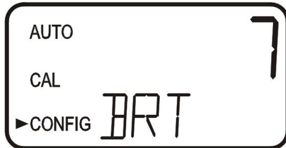
Change the brightness by pressing the  $\blacktriangle$  or  $\blacktriangledown$  button. When the desired brightness has been selected, press the  $\blacktriangledown$  button.
