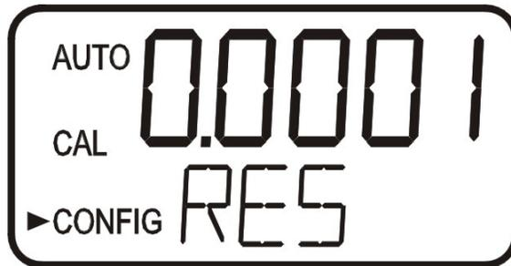
Change the resolution by pressing the  $\blacktriangle$  or  $\blacktriangledown$  button. When the desired digit resolution has been selected, press the  $\blacktriangledown$  button.
