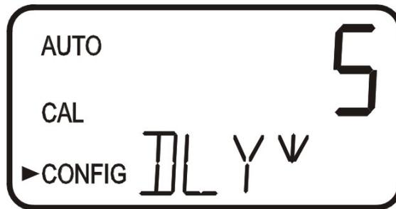
The current selected number of seconds will be shown. Select the desired delay off time for this alarm using the  $\blacktriangle$  and  $\blacktriangledown$  buttons. Once the desired delay time has been set, press the  $\blacktriangledown$  button to accept it. After the settings for alarm 1 have been completed, prompts will allow for the set up of the information on alarm #2.
