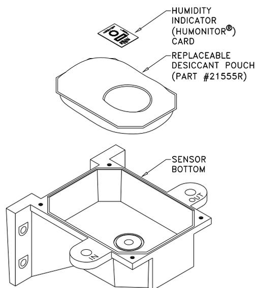
**Note:** Once the bag is opened, install the desiccant pouch immediately to prevent premature degradation of the desiccant.
