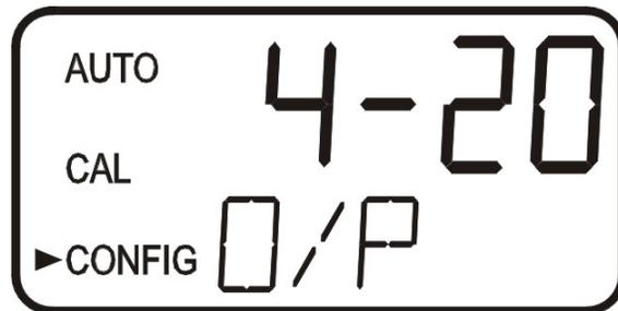
If the 4-20 mA output was turned on, prompts to set the 4mA (**4MA**) and 20mA (**20MA**) turbidity limits levels will be displayed. There is also a menu to adjust the error level (**ERLV**). The first prompt will be the turbidity limit assigned to the 4 mA output level:
