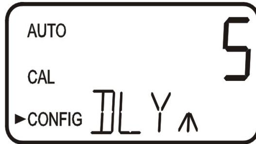
The current selected number of seconds will be shown. Select the desired number of seconds for the “delay on” time for this alarm using the  $\blacktriangle$  and  $\blacktriangledown$  buttons. Once the desired delay time has been set, press the  $\blacktriangledown$  button to accept it.
