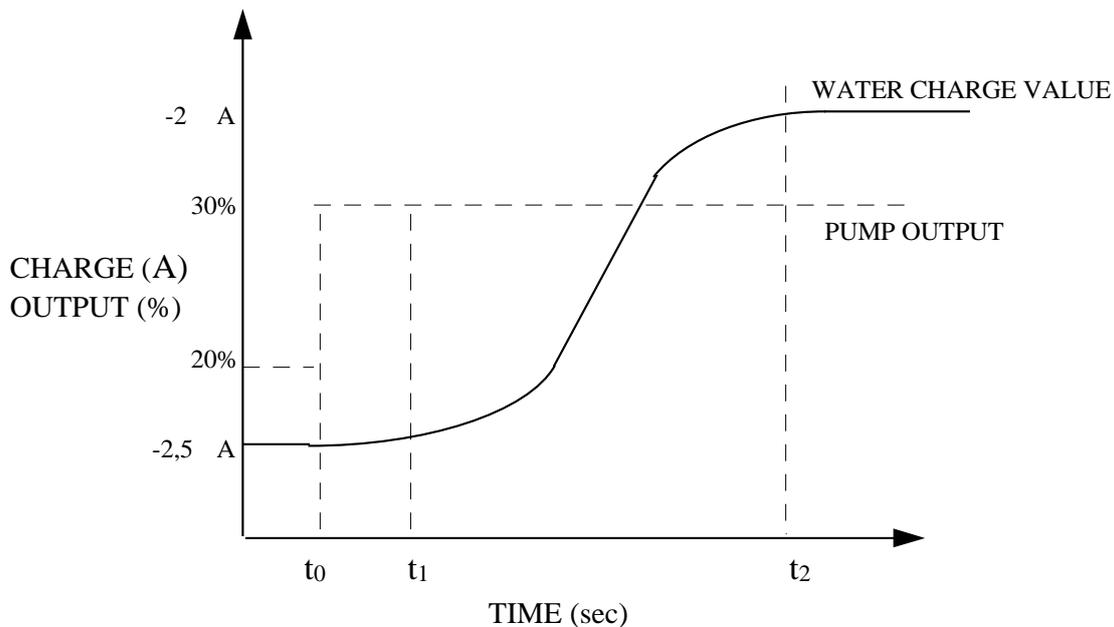
Figure 8. Dosage response curve to determine Proportional and Integral control constants.
