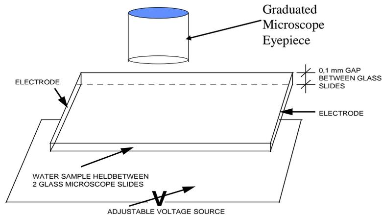
Figure 1. Measurement of Zeta potential using an applied electrical potential.
