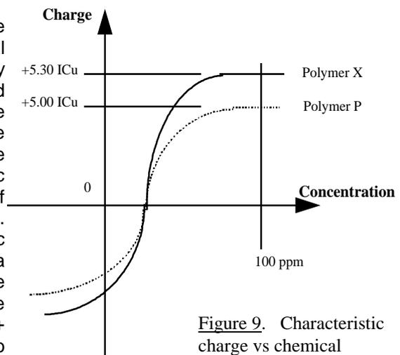
Figure 9. Characteristic charge vs chemical concentration curve for Polymer X and Polymer P
