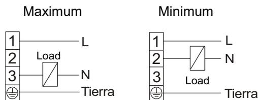
**NOTE:** The AC version has a power consumption of 6 mA when the load is deactivated. This should be taken into account when the load is a relay. You must make sure that the dropout voltage of the relay is greater than the voltage across the coil when a current of 6 mA flows through it. If the dropout voltage is equal or smaller then the relay can be in an activated position independent of the LD-61 state.
