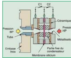
The differential pressure is applied to the silicon sensor and changes the two capacitance values (C1 and C2) of the sensor as a function of the measured pressure.
