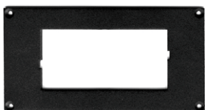
SMP-147/94 to mount 96 x 48 mm size unit in a place of 144 x 72 mm cut-out
